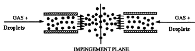
FIG. 1. Schematic diagram of a coaxial two impinging streams configuration.
